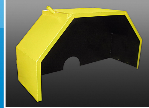
9. 水罩采用3mm厚钢板制作，内部采用沥青做防锈处理。 Blade Cover is made up of 3mm steel-plate, painted with asphaltum for anti-rust.
