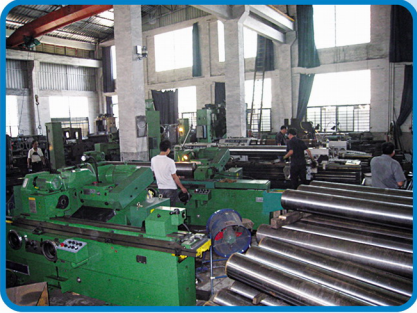
1. 采用全新磨床批量加工导柱，加工精度高，质量有保证。 Use CNC boring lathe to process the hole of sliding way column and headstock, to ensure the concentric and stability.
