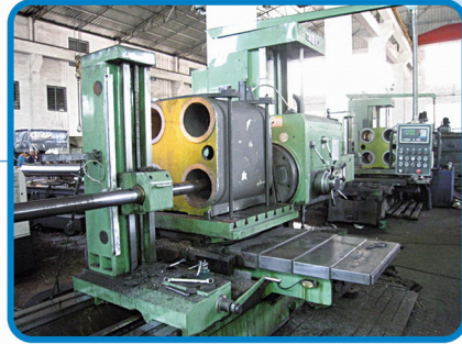
2. 采用数控磨床加工柱孔、主轴箱等，有效保证同心度的加工精度，提高产品稳定性。 Sliding ways of up/down system are quantity proceed by completely new grinding machine, for the purse of high precision and quality.
